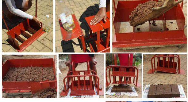
This block maker has been specially adapted to make goat blocks and is available from any hardware shop. (2019 price approx. R2300). Just ask for the HAKA Goat Block maker. If this maker is not available these blocks can be pressed by hand into plastic containers of appropriate size.
